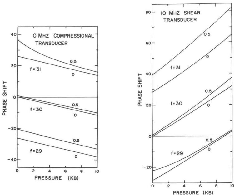
Fig. 6. (Left) Estimated effect of pressure on transducer-bond phase shifts for compressional [100] waves in  $MgF_2$  with a 10-Mhz quartz transducer. Curves are for  $\tau_f = 0$  and 0.5 nsec and carrier frequency  $f = 29, 30,$  and  $31$  Mhz. Bond properties are estimated (Table 3). Fig. 7. (Right) As in Figure 6 for shear waves.
