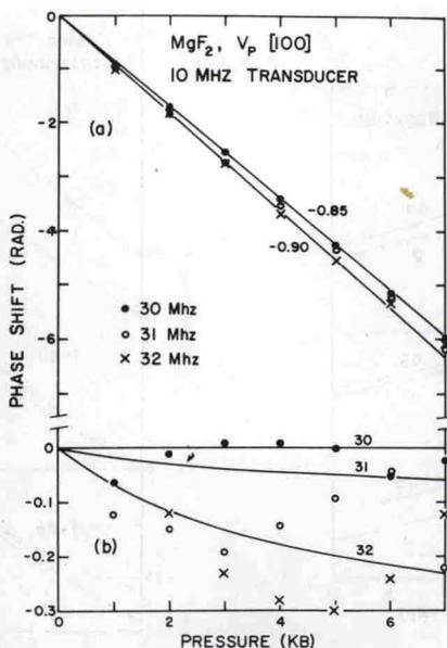
Fig. 8. (a) Measured phase shifts versus pressure (normalized to 30 Mhz) at 30, 31, and 32 Mhz for compressional [100] waves in MgF<sub>2</sub>. Lines are labelled with slopes (rad/kbar). (b) Residuals of measured phase shifts relative to line through 30 Mhz data, compared with calculated transducer bond phase shifts, assuming bond properties (Table 3) and  $\tau_f = 0.2$  nsec.
